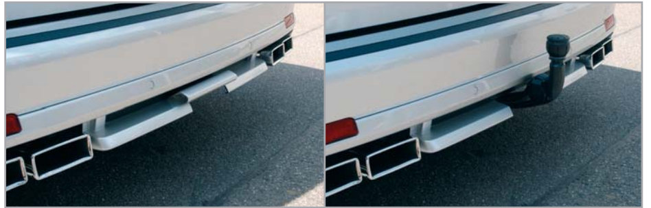
Dual branched twin-rear silencer i 34 08 044, rear lower skirt with parking distance sensor i 34 01 474 and cover i 34 01 462 for towing equipment. (Not pictured: rear lower skirt with parking distance sensor i 34 01 473 for rear silencer i 34 08 054 with twin tailpipes, left exit.)
